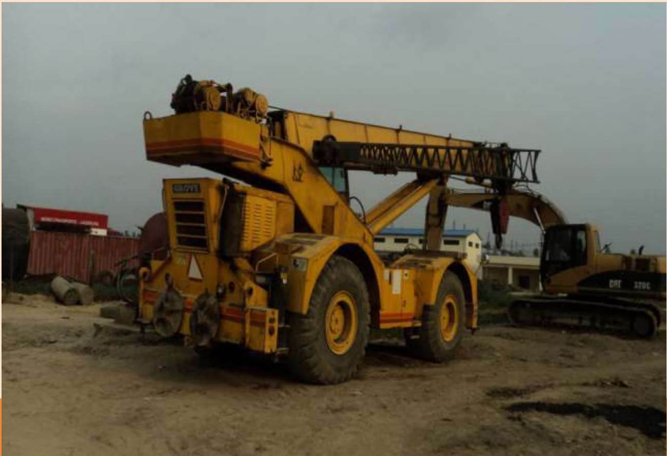
40Tons Grove Crane
